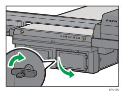
3. Open the cap of the ink tanks to be replenished with ink.
