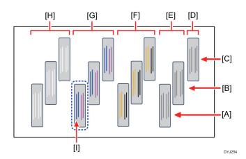
Symbol Description Symbol Description Print heads for Y/K nozzles Print heads for the first row (Head [A] [F] 1) [B] Print heads for the second row [G] Print heads for C/M nozzles (Head 2) [C] Print heads for the third row (Head [H] Print heads for W nozzles Print head for Pr nozzles [1] Reference nozzle (Cyan (Nozzle 1 [D] of Head 1)) Print heads for Cl nozzles [E]
