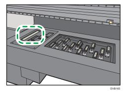
Remove the pad from the grooves located at both ends.
