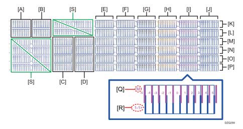
[A] and [B] are printed with primer ink. [C] and [D] are printed with clear ink. [E] and [F] are printed with white ink.
