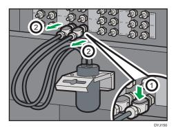
Pass the tubes through the holes of the air bubble ejection tool to avoid splashing the ink from the removed tubes.
