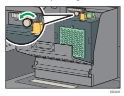
3. Slide the UV lamp to align the arrow with the value in Table 1.
