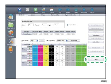
11. Print the test pattern again and check the adjustment pattern for all nozzles except for the reference nozzle.
