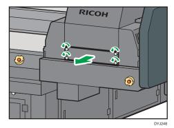
2. Attach the air bubble ejection tool at the maintenance station position.
