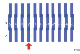
7. Enter the optimum adjustment value in [High] for [Bi-Direction Offset], and then click [Apply].
