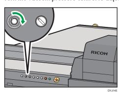
5. If the vacuum pressure is insufficient, turn the vacuum switch clockwise, and then adjust the vacuum pressure by using the vacuum pressure control.
