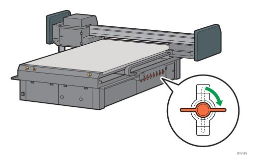
3. Turn the vacuum switch counterclockwise to vacuum the media.
