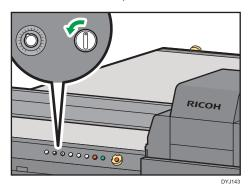
4. Turn the vacuum pressure control to adjust the vacuum pressure.
