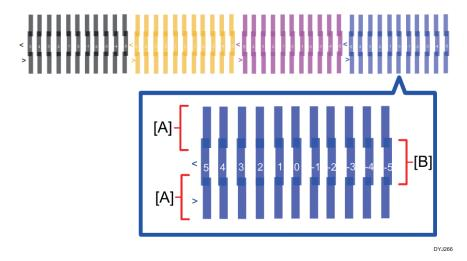
Find the pattern where outbound pass lines and return pass line are overlapped and aligned
