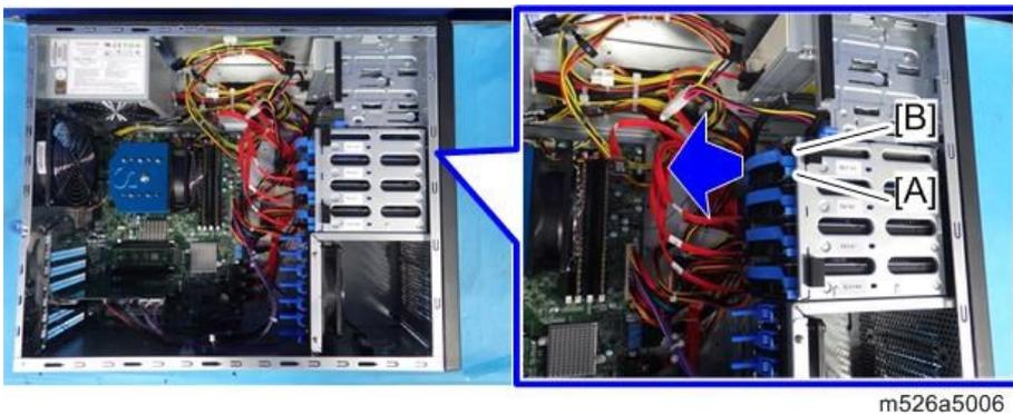
**4.** Remove the HDD [A]. (hook ×4)
