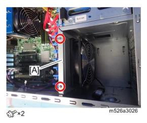
**4.** Remove the cooling fan [A] (rubber mount ×4).
