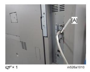
**2.** Connect the interface cable which is connected to the printer to the Gigabit Ethernet port (bottom) [A] of the print server.
