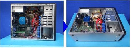
**<u>3.</u>** Cut the cable tie [A] fixing the power supply harness to the machine.
