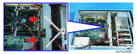
7. Remove the cooling fans with the bracket [A]. (5°×5)
