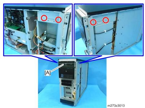
3. Remove the connectors that are connected to the DVD drive [A]. (\*\*2)
