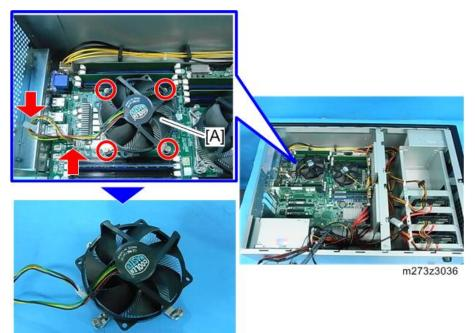
3. Unlock the upper/lower of the CPU socket [A].
