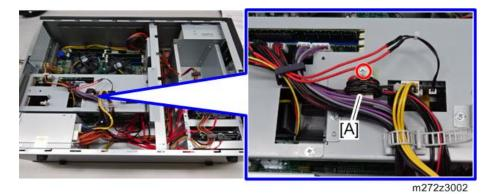
4. Release the ferrite core [A]. (@\*×1)
