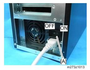
3. Push down the power switch (front side) of the print server.
