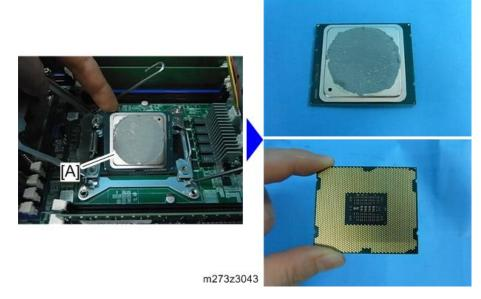
6. Grasp the edges of the CPU [A] and remove from the CPU socket.
