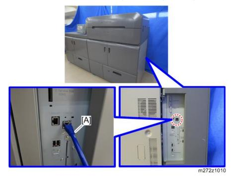
3. Connect the interface cable [A] to the Gigabit Ethernet port of the printer. (🕬 ×1)
