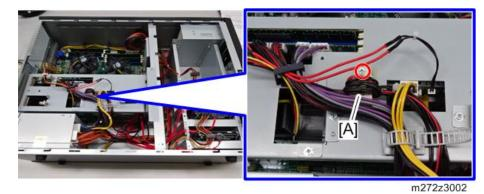
4. Release the ferrite core [A]. (SP×1)
