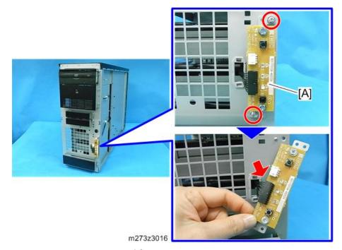
2. Remove the power supply SW board [A] with the bracket. (🕅 ×2, 😂 ×1)
