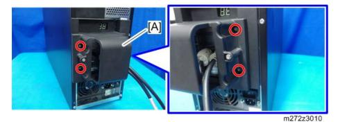
Remove the data transfer unit cables while pushing the lock behind the connector. (\*2)
