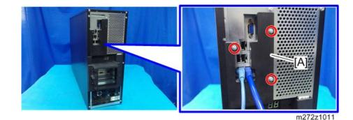
6. Connect the data transfer unit cable to the data transfer unit port [A] [B] of the printer.
