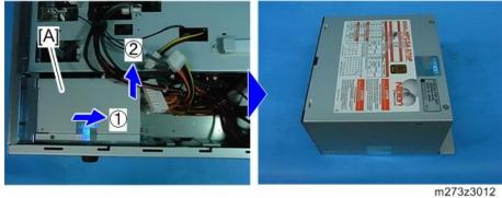
7. Remove the electrostatic tapes [A] on the PSU [B].
