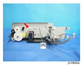
1. Disconnect the clutch harness [A] ( x 1).
