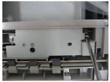
3. Set the paper end sensor in the correct position.
