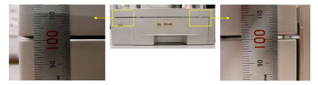
7. If the gaps are not within specification and even with each other, add a second Mylar on top of the first one, and repeat Steps 4 thru 6 until the requirements are met.
