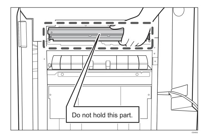
Holding this part can bend the entrance guide plate, or cause the connector for the sensor to become unplugged, which can lead to paper jams.
