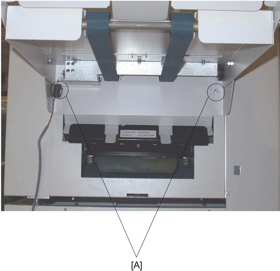
1. Loosen screws [A] to the Belt stacker (
