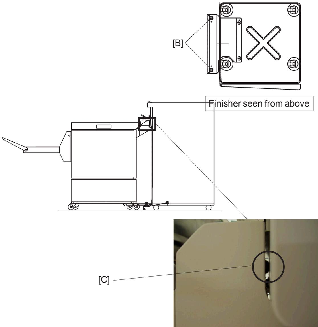
1. Loosen the two positioning pins [B] with the Multi tool.
