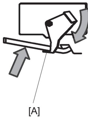
1. Remove the adhesive backing from the Exit arm catcher.
