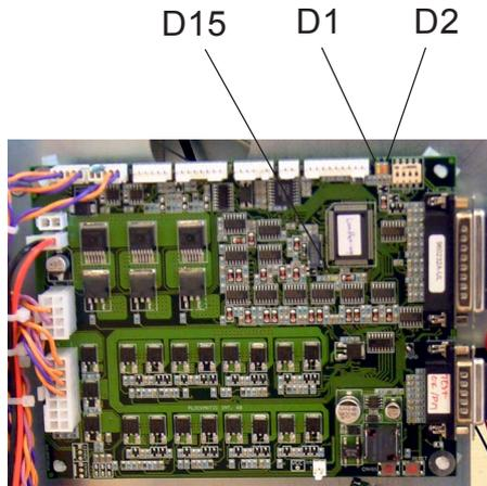
**D1:** Yellow LED flashes when power is on. The flashing indicates that a program is present and functioning. Should a download fail or the 5V be missing, LED would be OFF.
