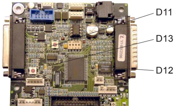
**D11:** Green LED is ON when power is switched on. At power up the 36V is checked that it is within allowed range. If within allowed range, LED illuminates and relay contacts closes for the 36V. If not within allowed range, LED stays OFF and relay will not let the 36V through.
