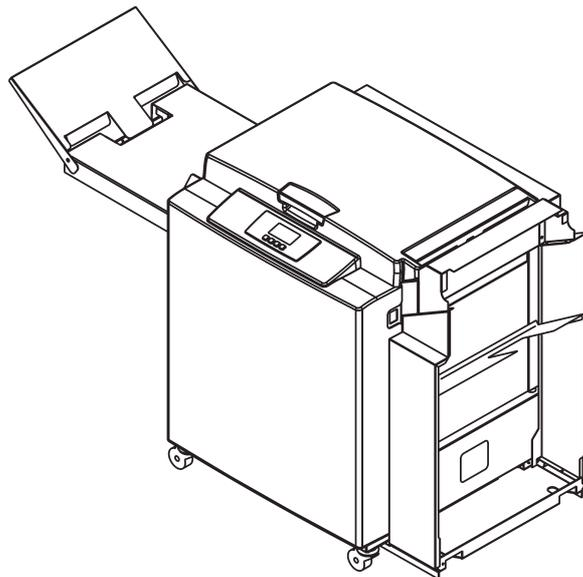
1. Remove all parts from the pallets. Slide the SR90 off the pallet, by pulling the two cardboard handles underneath the Booklet maker straight out [A].
