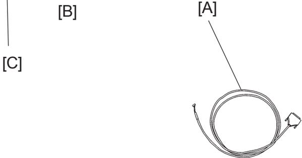
1. Install the Communication cable [A] from the installation kit, to connector CN132 on the finisher main board [B] (
