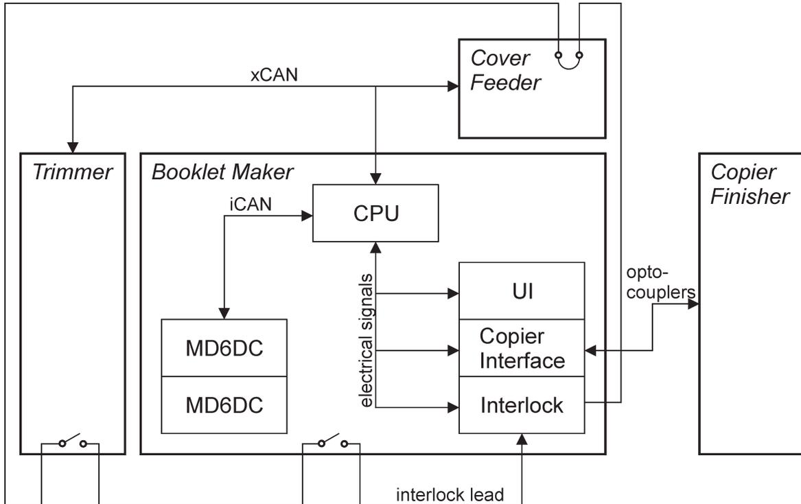
The electronics in the SR90 is distributed and divided in three different PCBs, one CPU board (CPU PCB PL76) and two motor drive boards (PCB MD6DC) . Each PCB has their own processor, they are communicating via internal CAN (iCAN). The system also has many support PCBs, such as one interlock PCB and one copier interface PCB.
