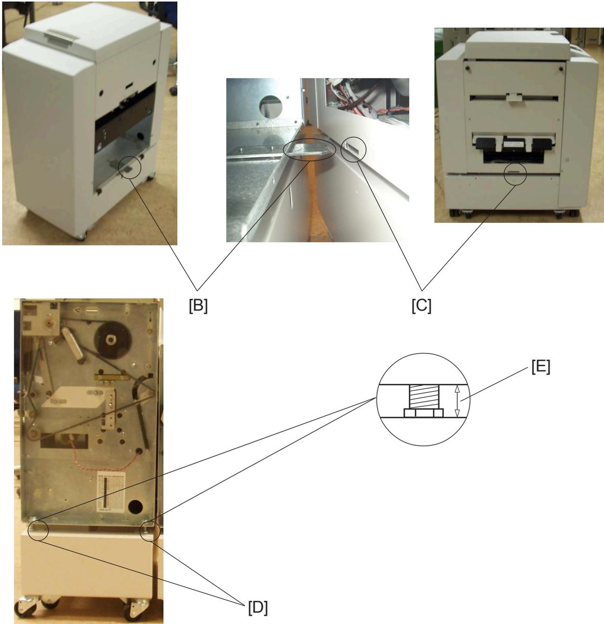
1. Remove the front cover by loosen two screws, and removing two screws (
