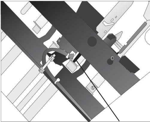
The sharp end of the tool on the 3rd stop finger.
