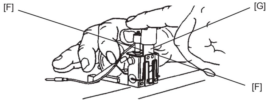
The stapler head drive post on each stapler head should be lubricated every 20 000 cycles.
