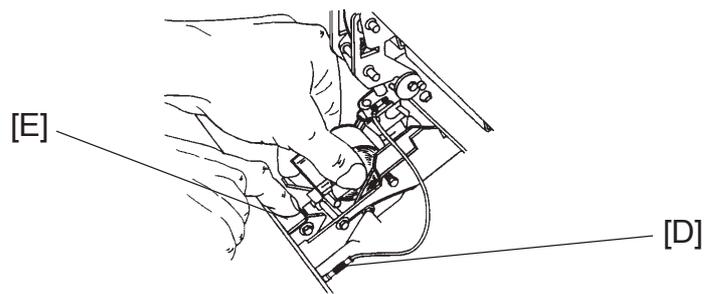
7. Disconnect the staple indication lead [D] from the socket.
