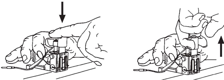
10. Remove staple cartridge. Look inside stapler head to locate jammed staples by eject point. Remove staples if any.
