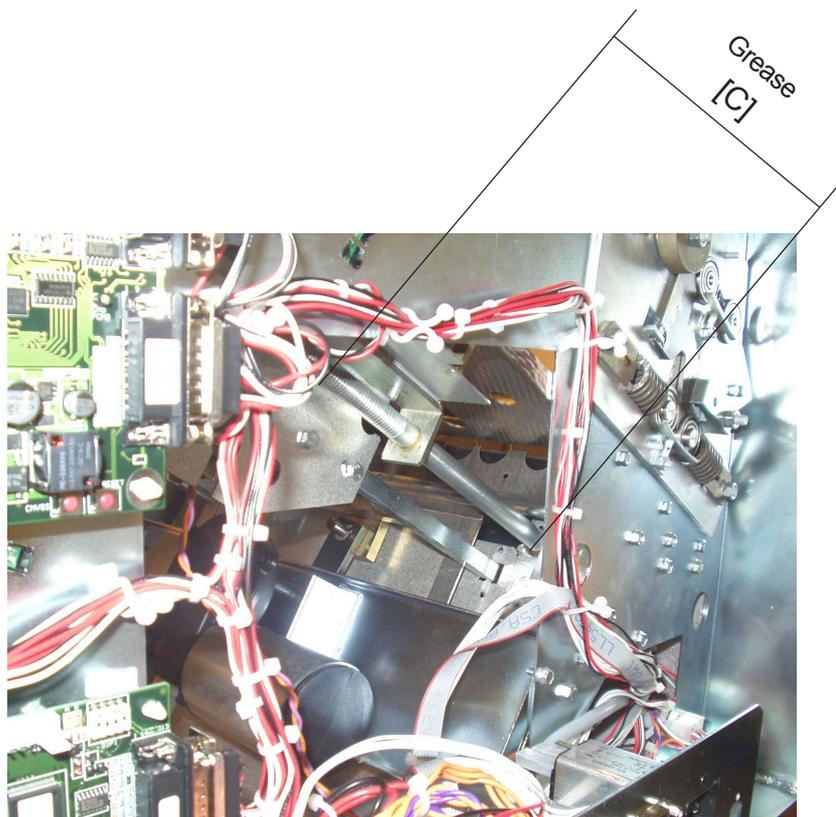
*View on Length adjustment shaft with Rear cover removed*
