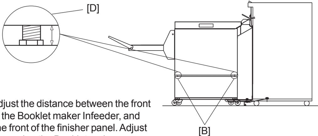
4. Adjust the distance between the front of the Booklet maker Infeeder, and the front of the finisher panel. Adjust by moving the Booklet maker.
