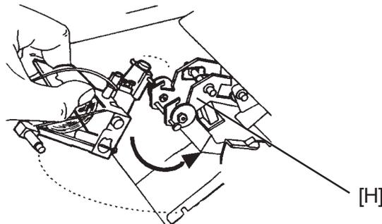
15. Reinstall the stapler head by inserting the pin at the top of the stapler head into the stapler retraction swing arm [H].
