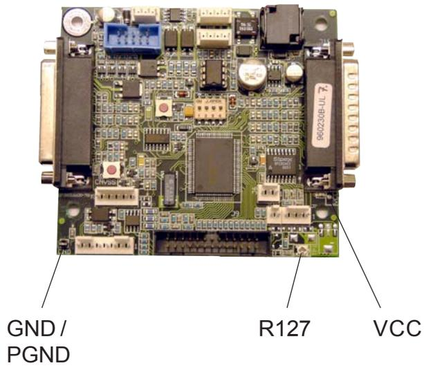
**VCC:** Stabilised and rectified 5V made from incoming 10V AC from transformer. Measure between Test Point VCC and Test Point GND/PGND using a voltmeter. The voltage will be shown on the voltmeter. Range 4.9-5.1V.
