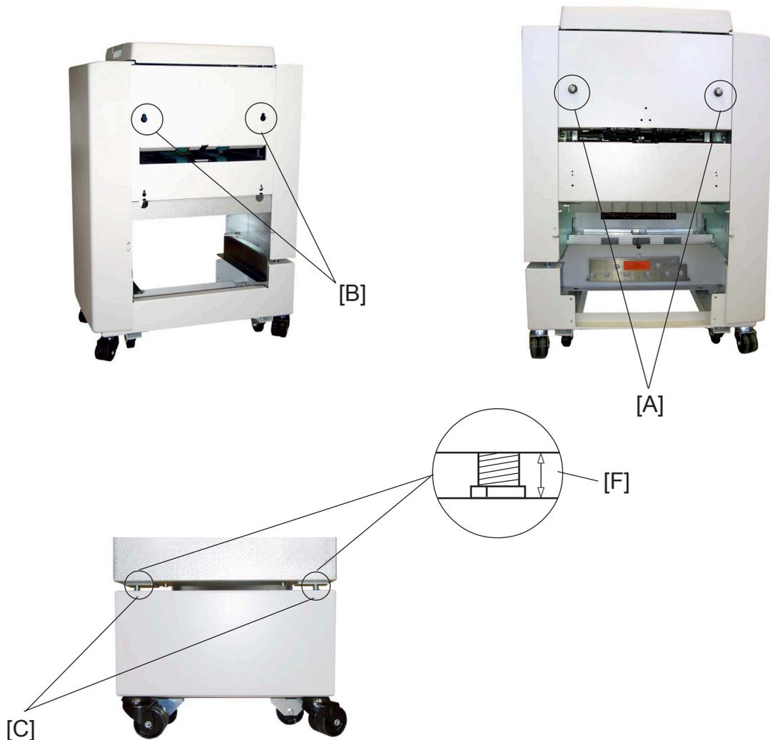
1. Remove the front cover of the Book Folder by removing two screws, and loosening two screws (
