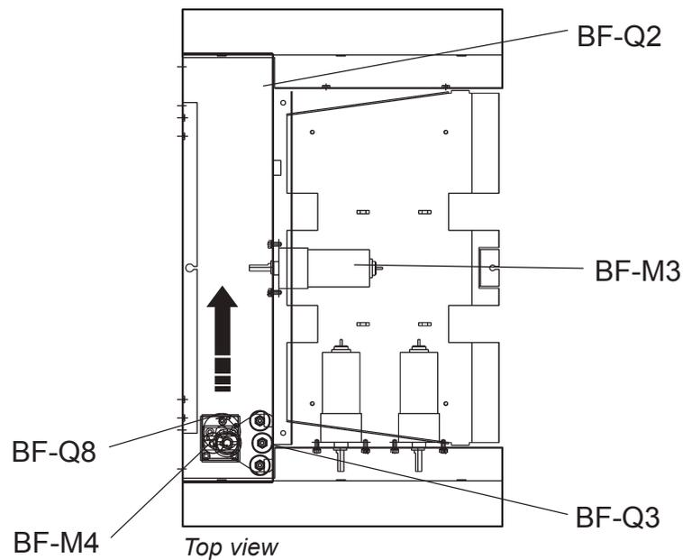
When Sensor BF-Q1 is deactivated, Roller motor BF-M4 is energized (moves (rolling) over the spine of the Booklet, pressing it up against the Set clamps, producing the Square fold look). The Encoder Sensor Q8 starts counting pulses by reading the Encoder Disc. When the correct number of pulses have been counted, motor BF-M4 slows down. When Sensor BF-Q2 or BF-Q3 is activated, motor BF-M4 stops.
