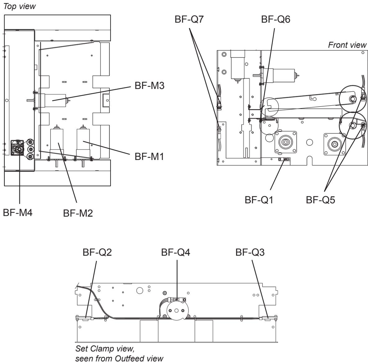
The BF90 performs an initialization-check at power on or when one of the interlocks has been opened and closed.
