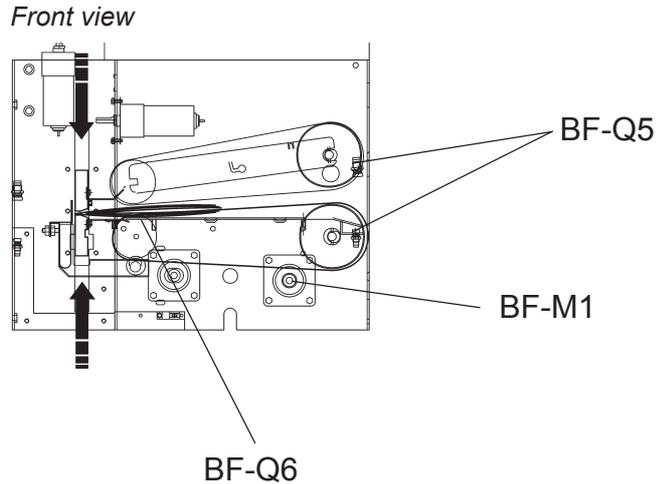
When Infeed sensor BF-Q5 is activated, the Transport belt Motor BF-M1 is energized. When Clamp sensor BF-Q6 is activated, Belt Stacker motor ST-M1 continues to feed out the set.
