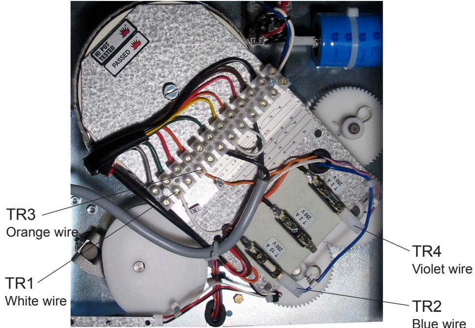
*Transformer in picture, tapped for 230V*
