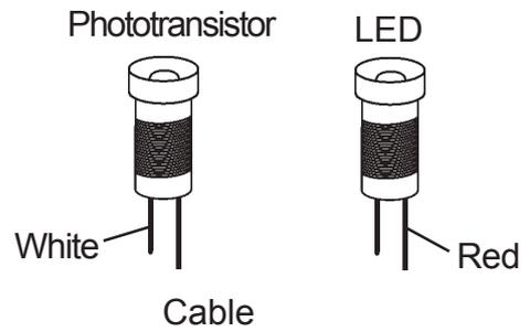
**Removal Q7 ,phototransistor**
