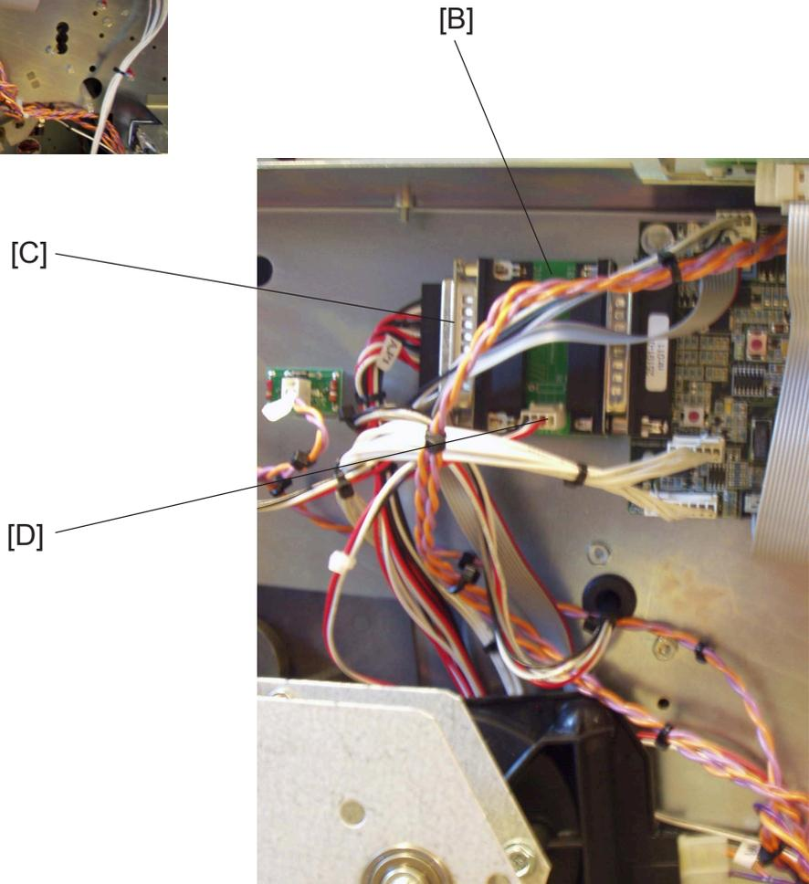
1. Remove the protection cover to the CPU PCB, by loosening two screws (
