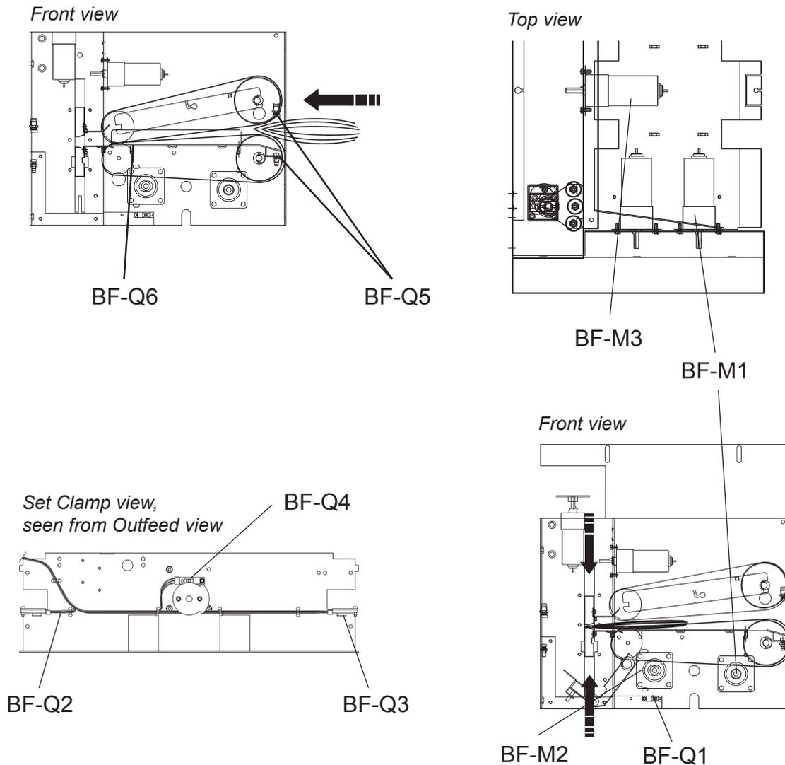
When Infeed sensor BF-Q5 is activated, the Transport belt Motor BF-M1 and Stop gate motor BF-M2 are energized, moving the Stop gate upwards. Motor BF-M2 runs until Stop gate sensor BF-Q1 becomes active, plus a certain amount of milliseconds. Motor BF-M1 Runs until Clamp sensor BF-Q6 is activated, plus a certain amount of milliseconds.
