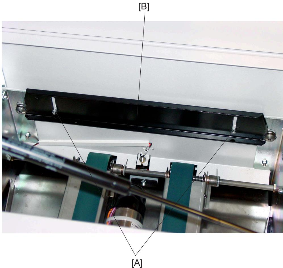
1. Loosen nuts [A] to the Locking bracket [B].
