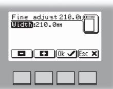
Press the [+] or [-] buttons to fine adjust in increments of 0.1 mm or 0.01 inches. Press the [OK] button to confirm.
