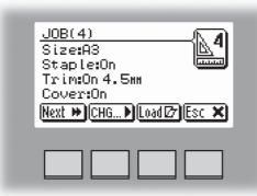
To recall a stored job press the [Jobs] button from the Ready screen to enter the Jobs screen. Select the desired job by pressing the [Next] button.
