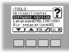
Select Software version with the [arrow] button and press the [OK] button. This screen, and sub screens show the software version for the different modules in the booklet making system.
