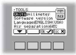
From this screen you can change units between millimeters and inches. Select Units with the [arrow] button and press the [OK] button.
