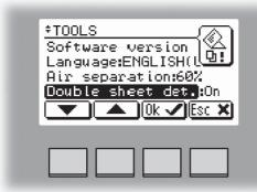
From this screen you can turn the double sheet detection On or Off. Select Double sheet det. with the [arrow] button and press the [OK] button.
