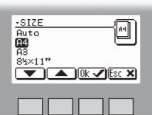
Select Auto or any standard paper size with the [arrow] button and press the [OK] button. Selecting Auto means that the booklet maker will automatically adjust to the same paper size (A4, A3, 8.5"x11" or 11"x17") as the copier.
