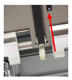
**2.** Insert the adjustment board (B4689003) between the jogger fences.
