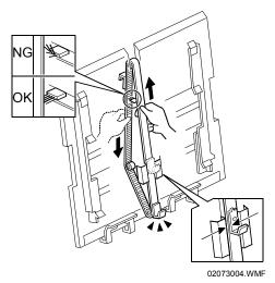
**20.** If the charge-removal brush is bent upwards, adjust it so that its fibers are perpendicular to the belt.
