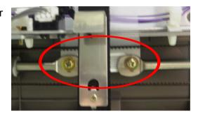
**5.** Rotate the R7 knob until the upper stay lightly contacts the adjustment board.
