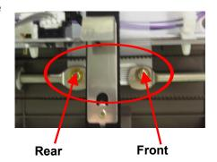
**9.** Tighten the screw for the rear jogger shaft all the way
