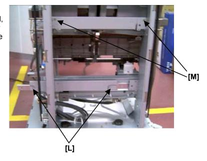
8. Secure the slide rail unit in place, then reattach all covers removed in the above steps.
