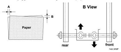
2) If C/D are over 2mm, **lower** the rear jogger fence shaft and re-secure the shaft in place. Then, loosen the screw for the front jogger fence shaft, **raise** the shaft to bring the front jogger fence flush against the paper, and re-secure the shaft in place.
