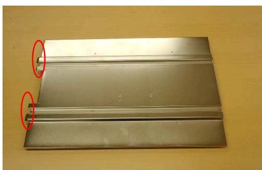
Countermeasure End Fence (Length of the end fence edges has been shortened to prevent contact with the roller.)
