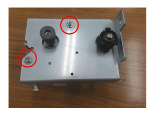
6. Remove the motor. (screw x2)
