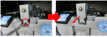
5. Remove the punch unit cover. (screw x2)
