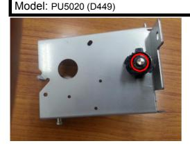
7. Remove the gear. (E-type retaining ring x1)
