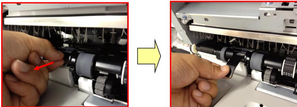
Pull out the guide plate at both front and rear at the same time
