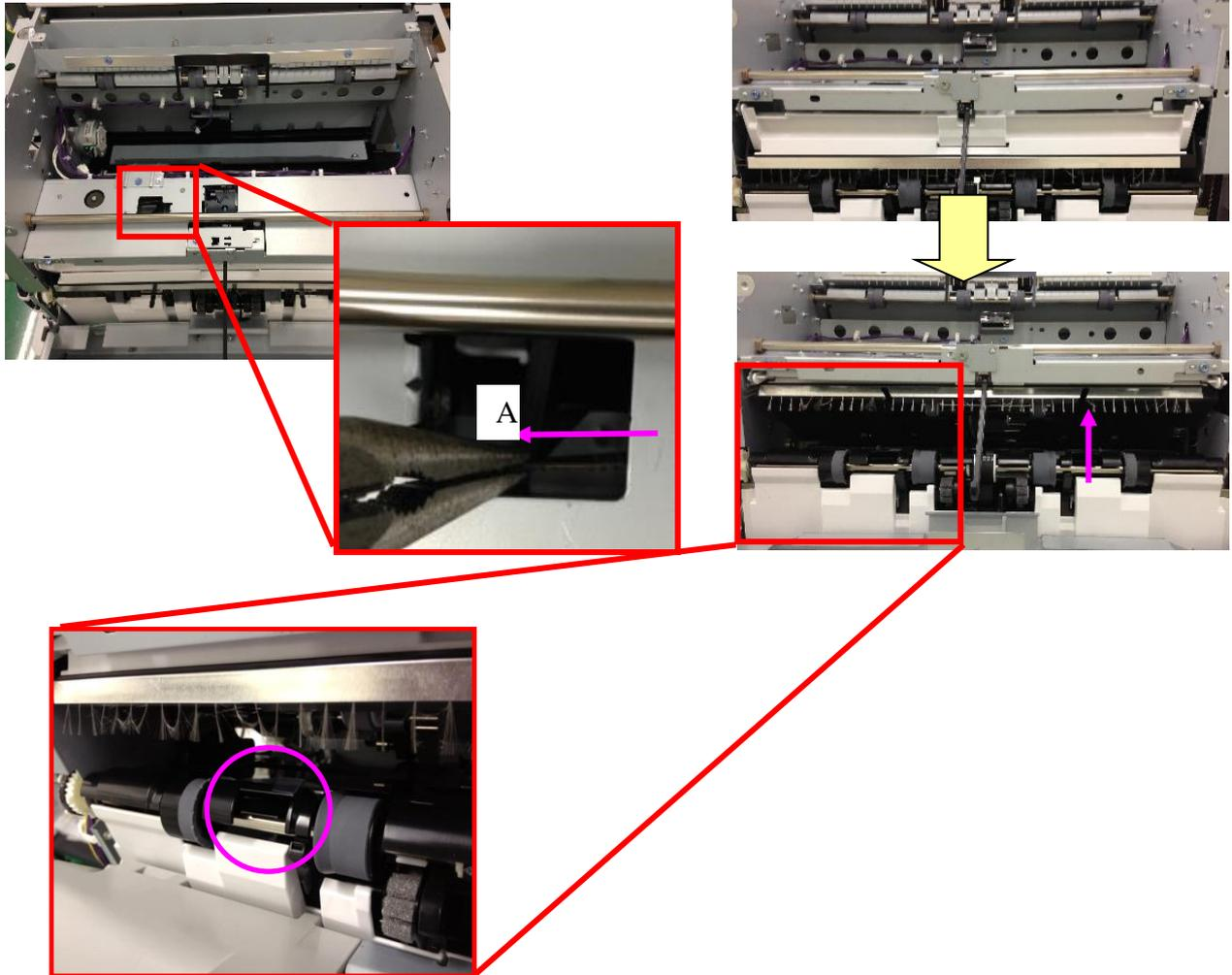
3. Pull out the guide plate (Front and Rear)
