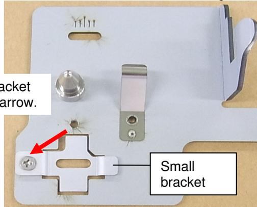
3-1. If the paper shifts forward (toward the operator side), slide the docking bracket by the same amount in the same direction. This is to move the finisher toward the operator side.
