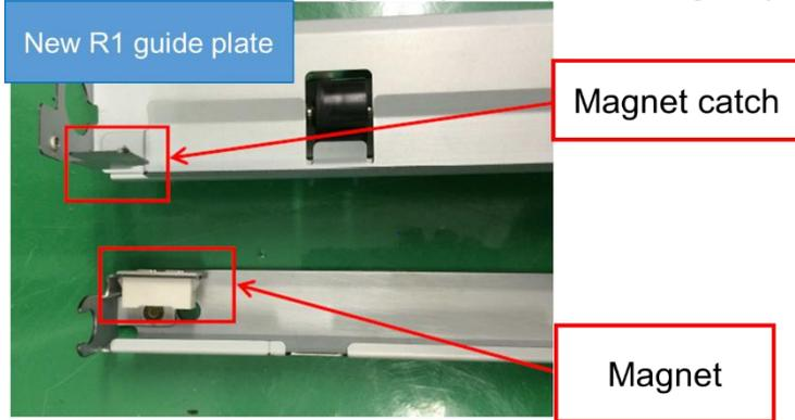
11. Open the R1 guide plate, locate the magnet at the rear side and confirm proper behavior.
