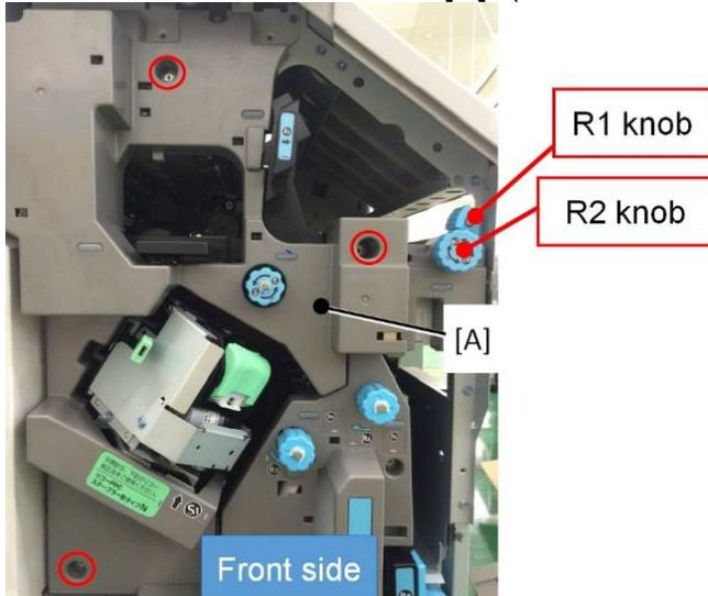
2. Remove two tapping screws, retaining ring, and bushing.
