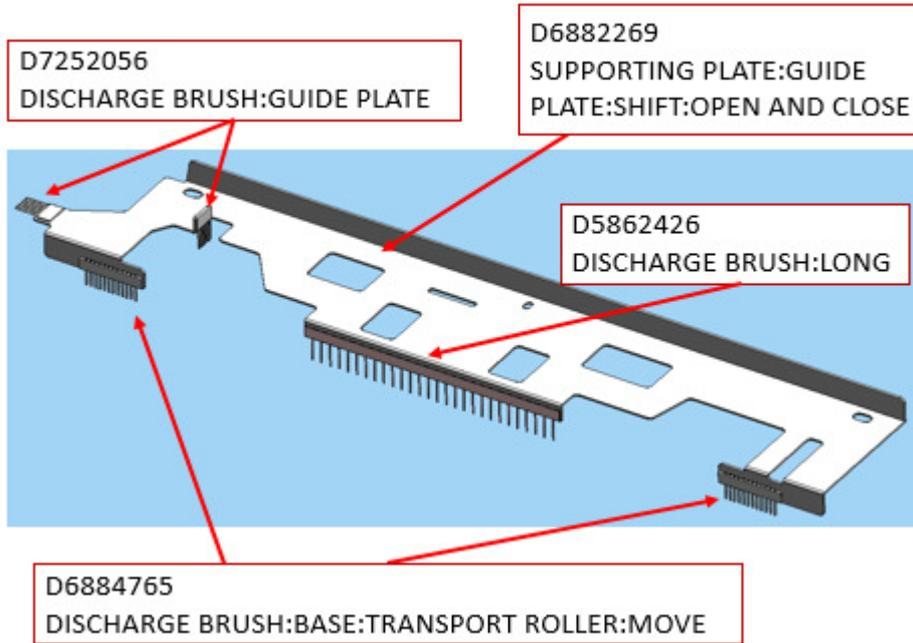
Discharge brush (p/n: D7252056) was attached to the gate pawl (p/n: D6882510).
