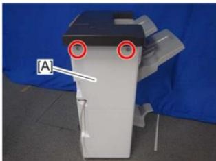
3. Open the front door [A] and remove the two screws for the upper cover (front) [B].
