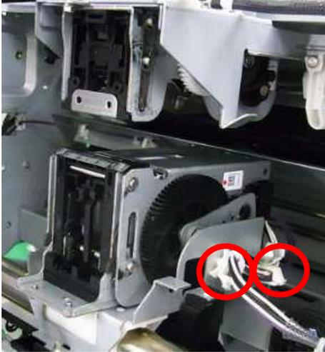
6. Remove the stapler drive unit [🔧 x 3].
