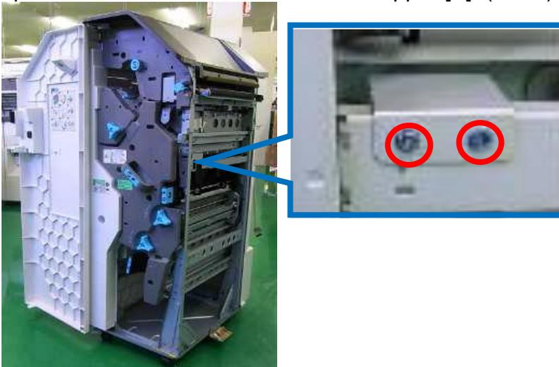
2. Pull out the staple folder unit and remove the guide. (🔩 x 2)
