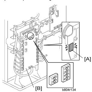
1. Read the DIP SW settings on the decal [A] attached to the back of the new folding unit.
