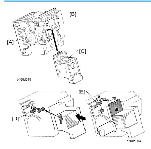
Staple firing is driven by the stapler motor [A] inside the stapler unit. The stapler hammer [B] fires the stapler [C].
