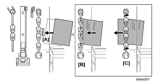
This punch unit corrects for paper skew and then positions the punch unit to punch holes at the correct position. Each sheet is punched one at a time.
