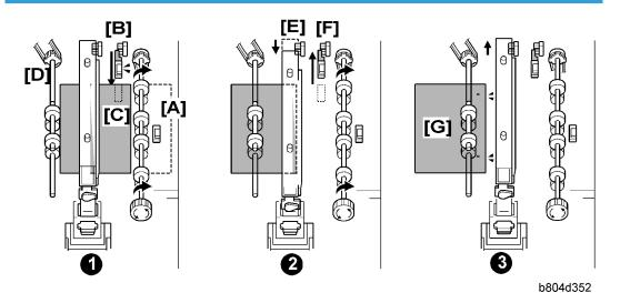
These operations (skew correction before punching, and punch unit position correction) increase the accuracy of the punch alignment.
