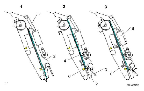
The last sheet of the stack [1] enters the stapling tray. The jogger fences [2] jog the last sheet into position (based on the width of the selected paper size) and then retract and stop 1 mm away from the sides of the stack.
