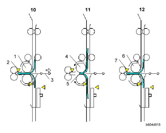
When the fold rollers [1] feed the stack 10 mm past the nip, the fold plate retracts until it no longer touches the stack. The fold unit exit sensor [2] detects the folded edge of the stack and stops the fold rollers.
