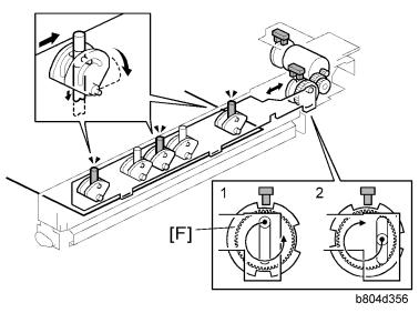
The timing for 2-hole punching [E] is different from 3-hole punching [F].
