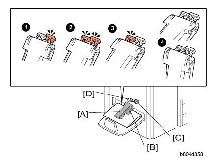
The lower tray sensor actuator arm [A] rests on the top of the stack of stapled booklets as they are output to the lower tray. A flap depressor [B] keeps the open ends of the booklets down.
