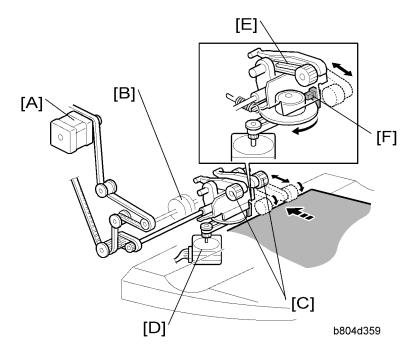
Upper/proof exit motor [A] drives feed roller [B] and stacking sponge roller [C].
