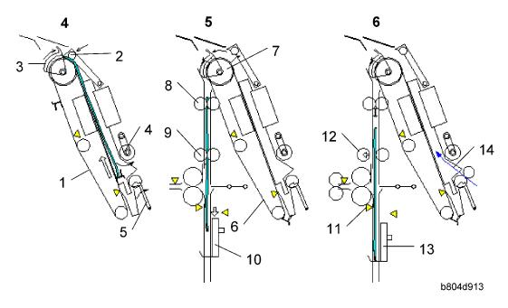
The jogger fences remain 1 mm away from the sides of the stack. The feed out belt [1] raises the stack until the top of the stack is 10 mm past the leading edge pressure roller [2] and stops. The leading edge pressure roller descends and applies pressure to the top of the stack. The stack junction gate [3] (normally open) closes. The pressure roller [4] and pressure plate [5] retract.
