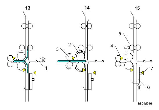
With the feed of the stack halted, the fold plate [1] retracts. The fold plate HP sensor (not shown) detects the fold plate and stops it at its home position.
