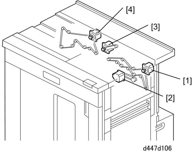
These are the motors that drive the rollers of the stacker:
