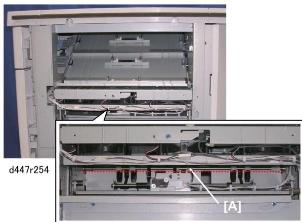
2. With the plate removed, you can see the paddle roller [A].
