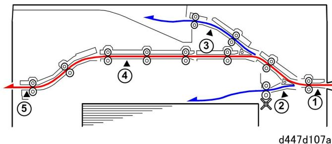
There are five main sensors at critical points in the paper paths. Each sensor detects the leading and trailing edge of each sheet of paper as it passes. If the paper fails to arrive (late error) or leave (lag error) within the prescribed time interval, the sensor will signal a jam.
