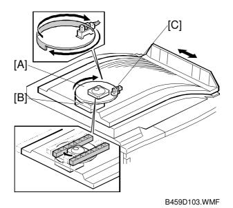
Half turn detection is performed through a combination of two components: the slip disc [A] and half turn sensor [C].
