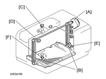
The lift motor [A] controls the vertical position of the tray through the timing belts [B].
