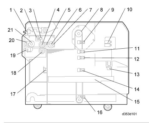
1. Rear LCT Set Switch 12. Sub Paper Height Sensor 2. Pick-up Roller Solenoid 13. Tray Down Switch 3. Tray Lift Sensor 14. Paper Height Sensor 3 4. Paper Feed Roller 15. Paper Tray 16. Lower Limit Sensor 5. Paper Feed Sensor 6. Paper End Sensor 17. Stack Sensor 7. Pick-up Roller 18. Separation Roller 19. Front LCT Set Switch 8. Tray Lift Motor 9. Paper Height Sensor 1 20. Relay Sensor 5 10. Interlock Switches 21. Relay Roller
