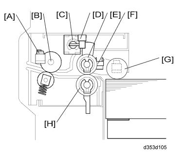
This machine uses the FRR paper feed system (paper feed roller [E], separation roller [H], pick-up roller [G]).
