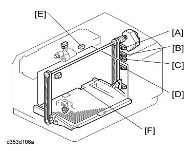
The amount of the paper in the tray is detected by combination of high (1)/low (0) outputs from three sensors (paper height sensor 1 [A], 2 [B], 3 [D] and sub paper height sensor [C]).
