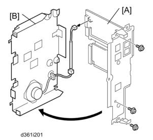
2. Separate the FCU [A] from its cover [B] (P x3, 🕬 x1).
