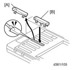
12. Remove the dummy keytop [A] (3rd from the top) and replace it with a facsimile keytop [B].
