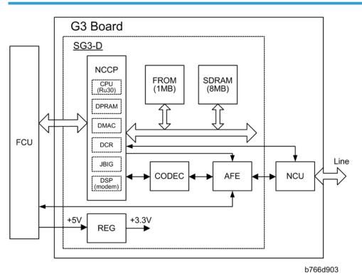
The SG3 board allows up to three simultaneous communications when used in combination with the FCU and optional G3 boards. The NCU is on the same board as the common SG-3 board. This makes the total board structure smaller. But, the specifications of the SG3 board do not change.
