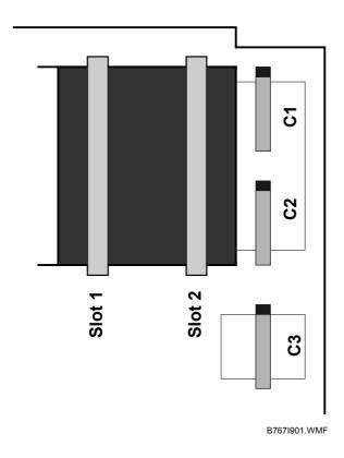
The names of the slots for the boards and SD cards are embossed on the face of the controller plate.
