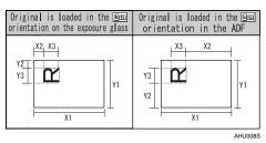
Specify [►Original Size] (X1 and Y1) using the number keys, and then press the [#] key.
