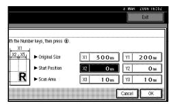
Specify [►Scan Area] (X3 and Y3) using the number keys, and then press the [#] key.
