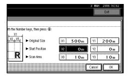
Specify [►Scan Area] (X3 and Y3) using the number keys, and then press the [#] key.
