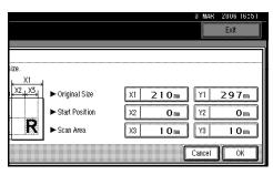
Set [►Start Position] (X2 and Y2) to 0 mm, and then press the [#] key.
