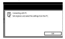
☐ Press **[Exit]** to use functions other than the network TWAIN scanner function.
