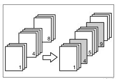
• Print on front side only Prints on the front side of the chapter slip sheets even if duplex printing is selected.
