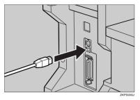
Plug the other end of the cable into the connector on the computer's interface.
