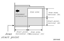
The maximum scan size is 432mm (17") in the Y direction (width) and 297mm (11.7") in the X direction (height). Keep the scan area settings within this range.
