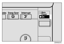
2 Turn off the main power switch to make the main power indicator go off.
