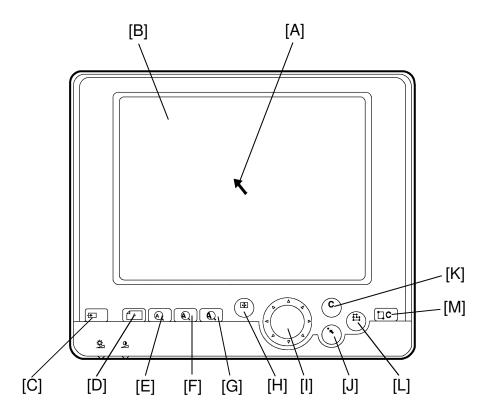
The scanned image is sent to the display editor and displayed on the LCD (640 x 480 dot).
