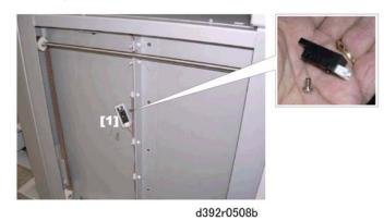
2. Remove the sensor [1] ( $\mathfrak{L} \mathfrak{I} \times 1$ ,  $\mathfrak{F} \times 1$ ).
