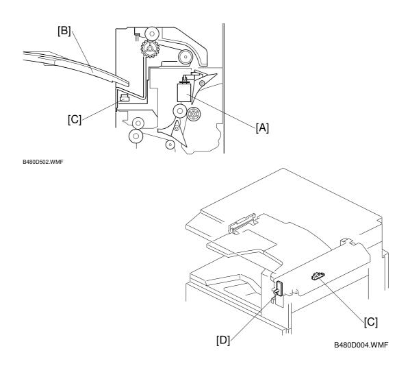
At the appropriate time after the leading edge of the first sheet of copy paper reaches the copier's registration roller, the junction gate solenoid [A] in the interchange unit turns on to switch the junction gate to direct the paper to the tray [B].
