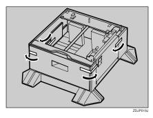
Adjust the four corners of the printer to those of the 2000sheet Large Capacity Tray, and then slowly lower the printer into place.
