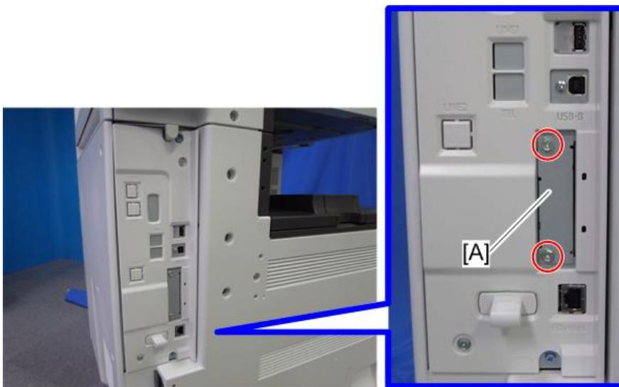
1. Remove the slot cover [A] from the board slot (⚠ x 2).
