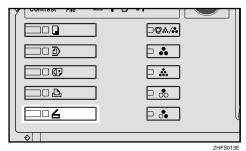
If user codes are set, enter a user code (consisting of up to eight characters) with the number keys, and then press the [#] key.
