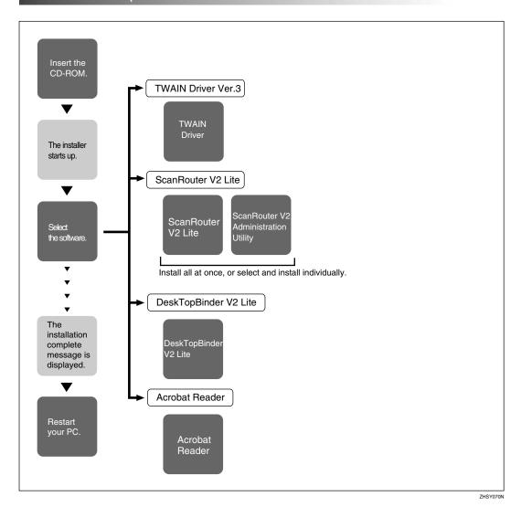
For information about the outline of the software that can be installed by Auto Run, see p.38 "Software Supplied on CD-ROM".
