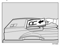
**3** Select the appropriate orientation so that it matches the orientation of originals placed.
