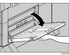
**11** Hook the mounting bracket to the hole, as shown.
