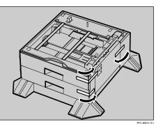
Adjust the four corners of the printer to those of the 1000sheet paper feed unit, and then slowly lower the printer into place.
