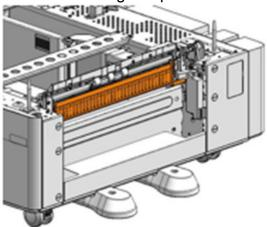
2. Remove the double tape from the guide stopper.
