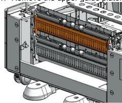
2. Remove the auxiliary guide plate for the "lower paper guide:lower" (screws x1).
