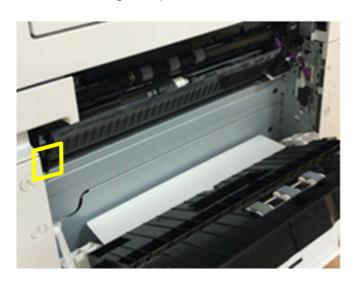
2. Attach the guide plate by sliding it toward the right hole.
