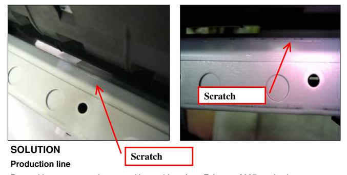
Parts without any scratch are used in machines from February 2007 production.
