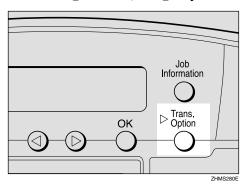
Press the ② or ⑤ key to display "9. Transfer Request", and then press the [OK] key.
