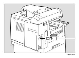
Plug the other end of the cable into a hub.
