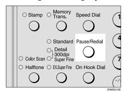
The last 10 destinations you dialed are shown. Press the ③ or ⑤ key to display the destination which you want to deliver the scanned data to.
