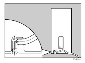
Connect the cable from the 4-bin mailbox to the lower connector on the back of the printer.
