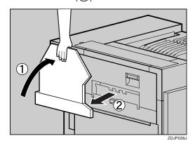
If the duplex unit is installed, open the duplex reversal unit.
