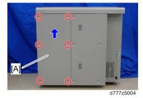
2. Lift the rear left cover [A] of the vacuum feed LCIT and remove it (@x10).
