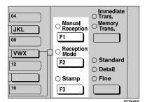
Confirm that "1. SUB" is displayed and press the [OK] key.
