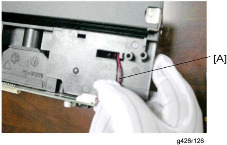
5. Turn over the scanning unit to disconnect the lamp inverter cable [A].
