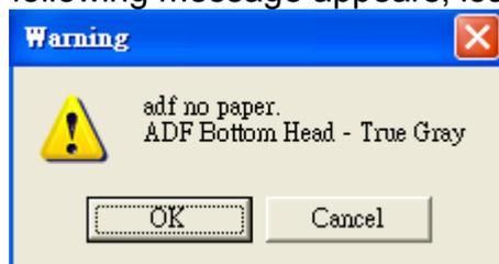
11. If the following error message appears, the test chart is loaded in the ADF in the wrong direction.
