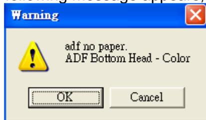
10. When the following message appears, load the test chart in the ADF and press **OK**.
