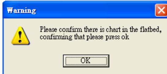
9. When the following message appears, load the test chart in the ADF and press **OK**.
