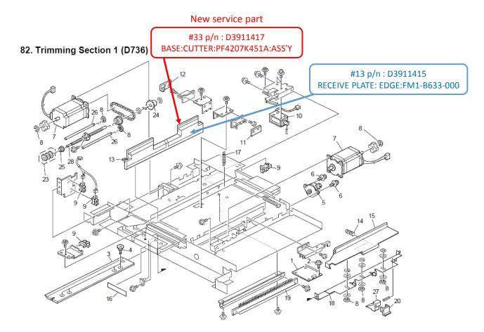
The new service part (p/n: D391 1417) attaches to "RECEIVE PLATE: EDGE:FM1-B633-000" (p/n: D391 1415).
