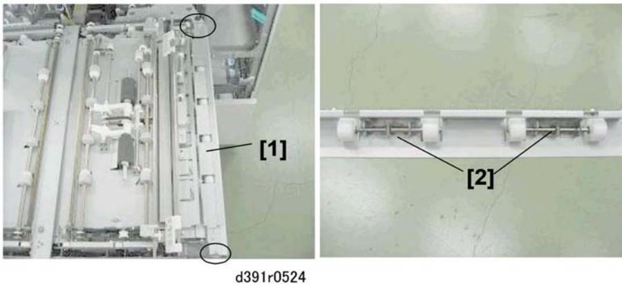
1. Remove the horizontal transport roller 1 idle roller unit [1] (⚙️ x2).
