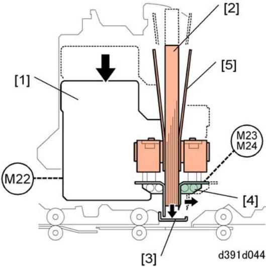
The main grip lift motor (M22) turns on and lowers the main grip unit [1] and signature [2] as far as the signature guide plate [3].
