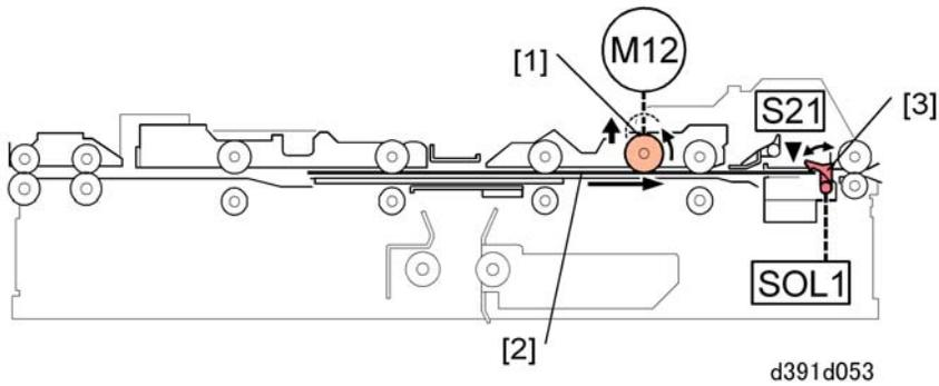
The cover motor: right (M12) reverses and rotates the buffer roller [1] at 500 mm/s and feeds the cover [2] toward the switchback position. The cover is fed to a position at a prescribed distance away from the cover registration sensor (S21) then the motor stops. This is the cover vertical position ("vertical" means "direction of paper feed").
