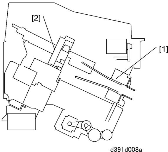
The main grip unit [1] receives the signature from the sub grip unit [2], tamps the spine of the signature to align it for gluing, lowers the signature onto the gluing unit for the application of glue to the spine, and then passes the signature to the trimming unit.
