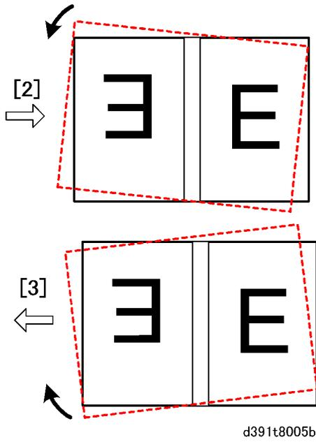
5. Do some test prints and then repeat the adjustment until the cover and signature are correctly aligned.
