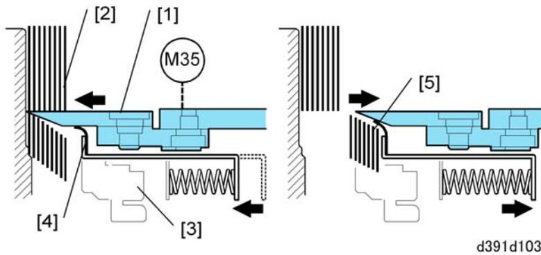
The cutter motor (M35) turns on and drives the blade [1] against the edge of the book [2] to perform the cut. The trimmings catcher [3] and the trimmings seat [4] move with the blade when it performs the cut.
