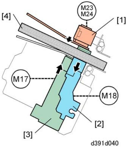
The grip motor: front (M24) and grip motor: rear (M23) switch on and close the main gripper [1] to clamp the signature tightly at the spine. Next, the sub grip motor (M20) turns on and opens the sub gripper [2] to release the signature in the sub grip unit. After the signature is released by the sub grip unit [3], the sub grip lift motor (M17) turns on and raises the sub grip unit about 5 mm away from the signature [4], then returns the sub grip unit to its home position.
