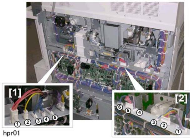
3. Disconnect connectors at [1] (🔌 x5) and [2] (🔌 x6).
