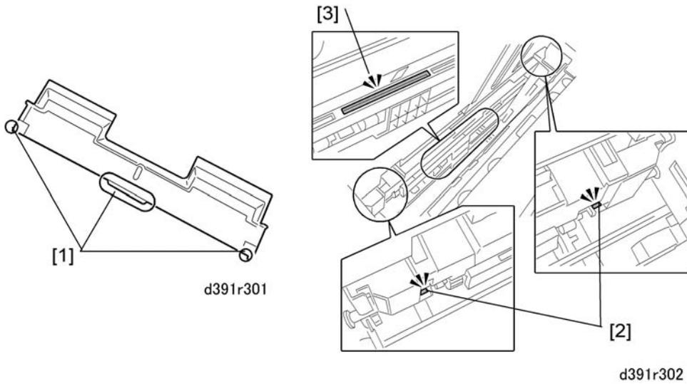
1. When reinstalling the blade cradle confirm that the three pawls [1] of the cradle are inserted in the holes of the trimming unit [2] and locked in the groove [3].
