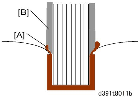
If there is an excessive amount of glue present when the signature and cover are joined, or when the three edges are trimmed, glue seepage at the corners could transfer from the signature [A] to the main grip [B] and interfere with operation. For this reason the amount of glue applied to the spine always must be within the ranges described above.
