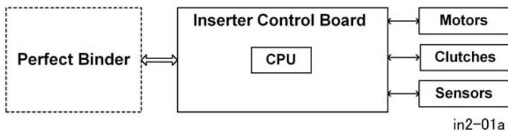
The inserter control board and its CPU (IC7) control the operation of the inserter unit. The CPU reads and interprets the input signals from the bookbinder and the inserter sensors. The CPU uses this information to run the inserter motors and clutches according to pre-set timings. The inserter is supplied with DC 24V power from the bookbinder. The inserter control board communicates with the sensors through serial connectors and harnesses.
