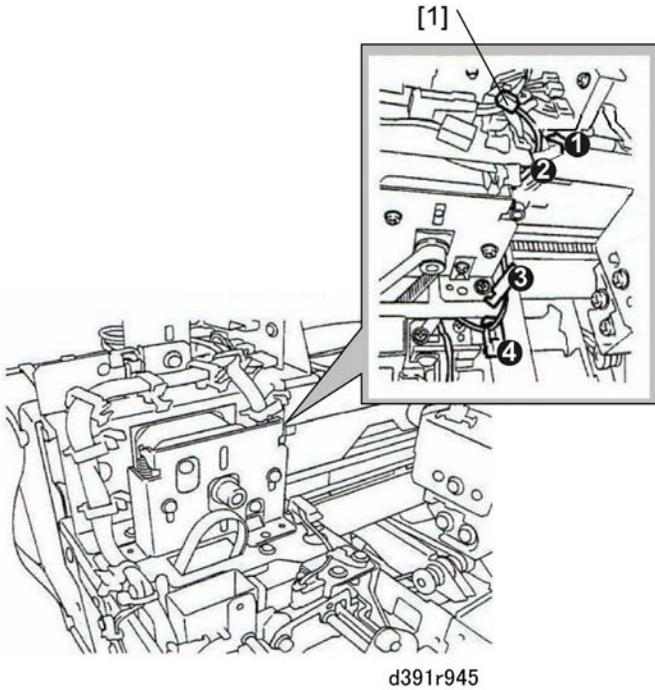
16. Release the thermistor harness [1] at the front side of the glue heater unit (
