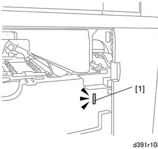
4. Insert piece of cardboard or folded piece of paper into the left door switch slot [1].
