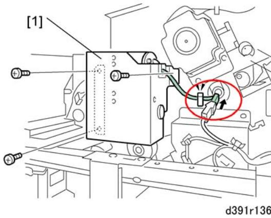
6. Remove the protection plate [1] (🔧 x1, 🛠️ x1, ⚙️ x3).
