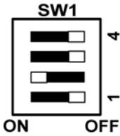
2. On the inserter control board set the DIP SWs as shown above.
