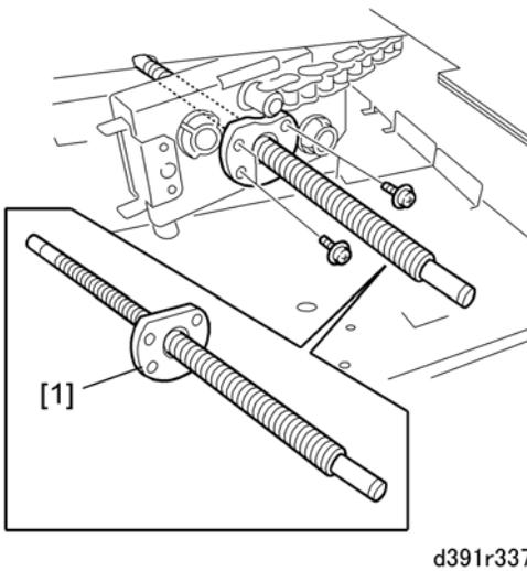
16. Remove the ball screw [1] (⌀ x4). If it is difficult to remove, rotate the shaft.
