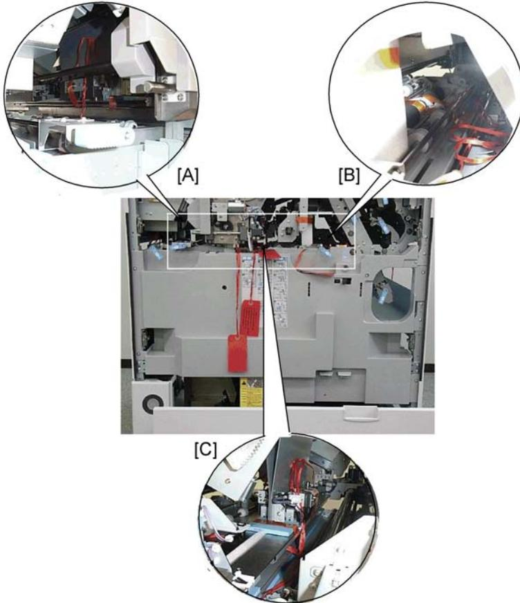
1. Remove the strips of tape and cushions from the horizontal transport unit at the left [A], right [B], and center [C].
