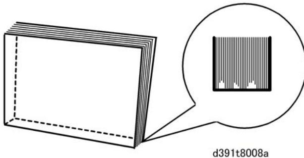
The distance set for switchback alignment during signature jogging in the stacking tray is not correct.
