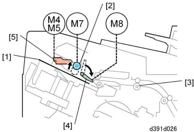
After the leading edge of the paper [1] is detected by the timing sensor (S5) and after the paper has traveled the prescribed distance, the switchback roller lift motor (M7) turns on. This lowers the switchback roller [2] to the transport position and the paper feeds into the nip of the switchback roller.
