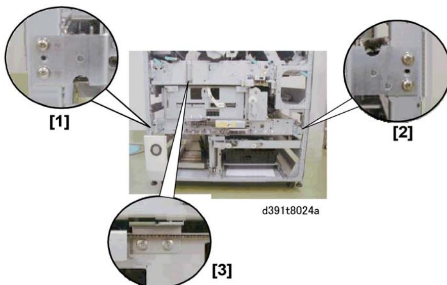
4. Remove the braces [1], [2], [3] from the trimming unit frame. (🔧x3 ea.)
