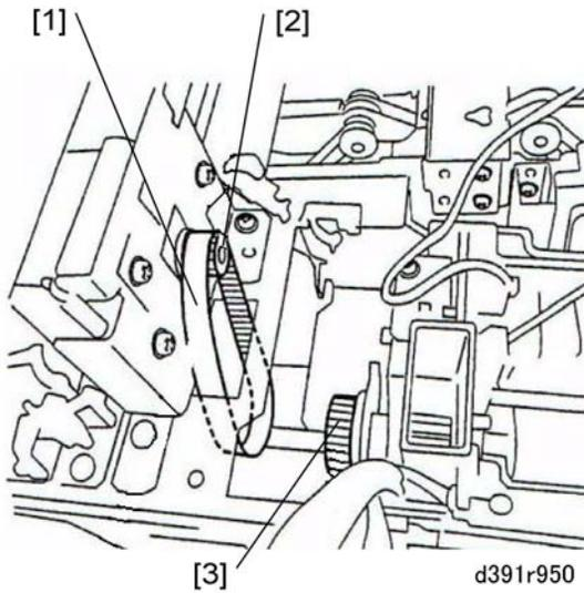
1. Reconnect the timing belt [1] to the motor drive gear [2] and shaft gear [3].
