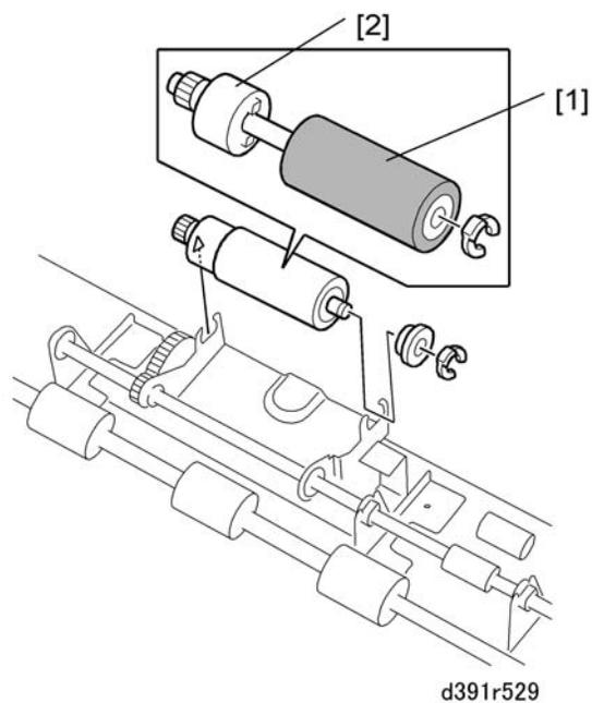
4. Remove the separation roller [1] (☛ 1, Bushing x1)
