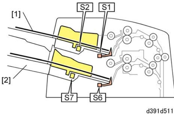
Tray A [1] and Tray B [2] are both provided with one paper set sensor (S1 (INS) for Tray A, S6 (INS) for Tray B) to detect the presence of paper on the trays.
