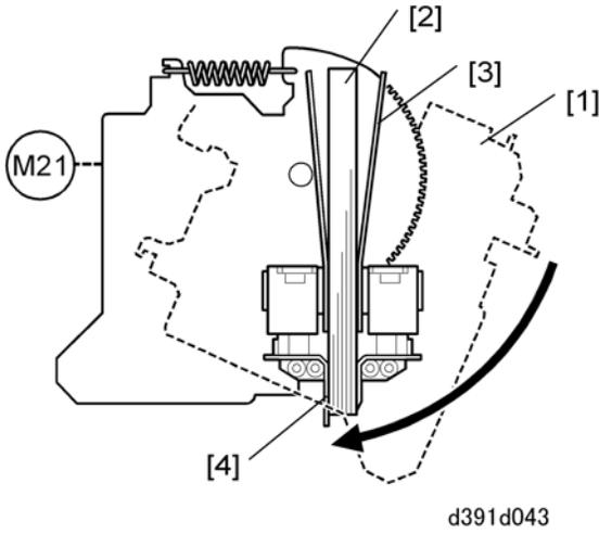
The grip unit rotation motor (M21) turns on and rotates the main grip unit [1] with the signature [2] clamped by the mini-gripper [3] and main gripper [4].
