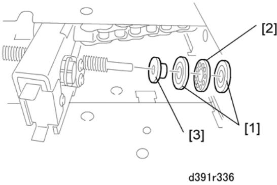
15. Remove the rings [1], bearing [2], and bushing [3] from the end of the ball screw.
