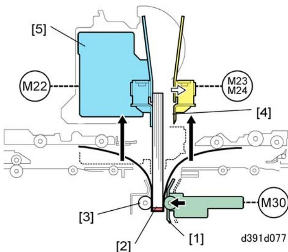
The signature path exit motor (M30) turns on, pushes the signature exit guide [1] to the left and lamps the signature and cover [2] in the nip of the signature exit rollers [3].
