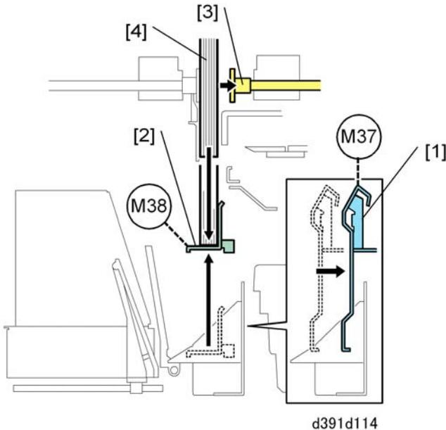
The trimmings buffer motor (M37) turns on and retracts the book press plate [1] in the transport path.
