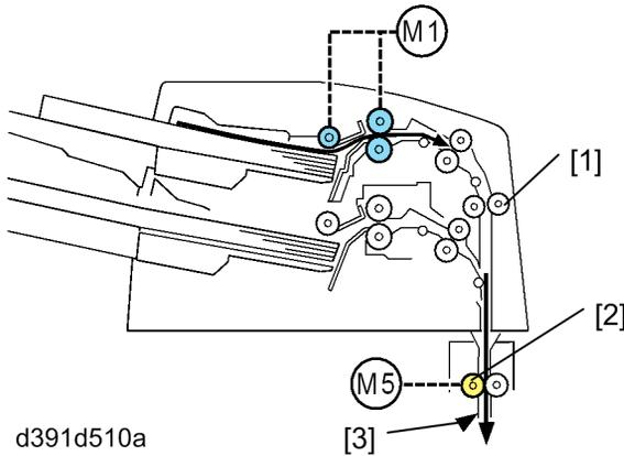
Once the sheet in the feed path has fed 20 mm past transport rollers 1 [1], the tray feed motor (M1 (INS)) stops and then reverses to start feeding the next sheet. If another sheet is not available, the tray is lowered. When vertical transport sensor 1 (S19 (INS)) detects the passage of the trailing edge feeding into the vertical transport roller 1 [2] this signals the vertical transport motor (M5 (INS)) to turn off.
