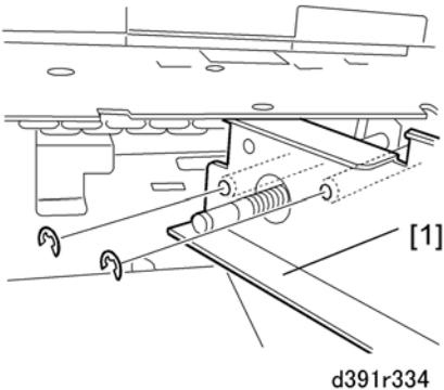
13. Remove the motor frame [1] (🌀 x2).
