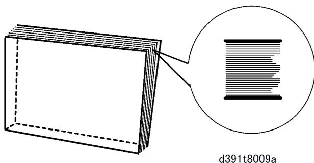
The front and rear jogger fences are not aligning the sheets during the jogging operation in the stacking tray as each sheet arrives in the tray.
