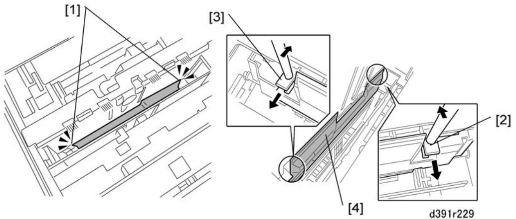
16. At the front and rear [1] insert a screwdriver at [2] and [3], press in the direction of the arrows to release the pawls of the blade cradle, then remove the blade cradle [4].
