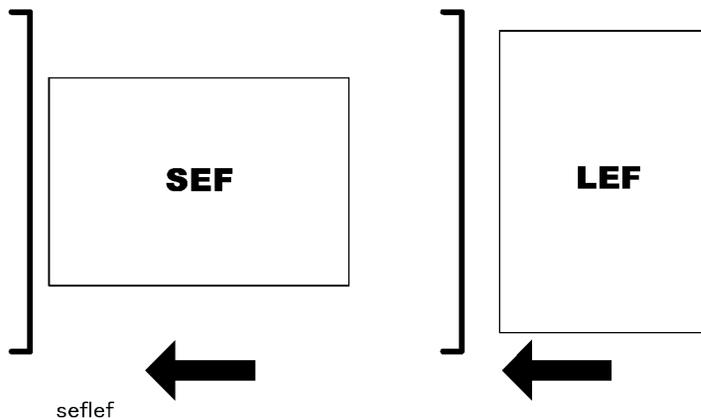
The notations "SEF" and "LEF" describe the direction of paper feed, with the arrows indicating paper feed direction.
