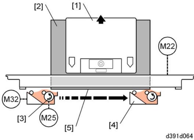
The main grip lift motor (M22) turns on, raises the main grip unit [1] and signature [2] slightly higher. Also, the glue vat roller motor (M25) turns on and reverses the rotation of the glue vat roller [3].
