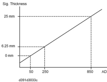
The signature thickness sensor (S50) measures the thickness of the signature the first time the grip unit closes onto the signature. A corresponding AD value is stored in EEPROM for mm readings from 0 to 25 mm as shown above.
