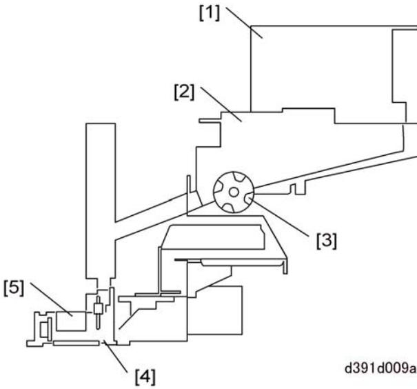
The gluing unit applies glue to the spine of the signature that will be joined with the cover to form the book.
