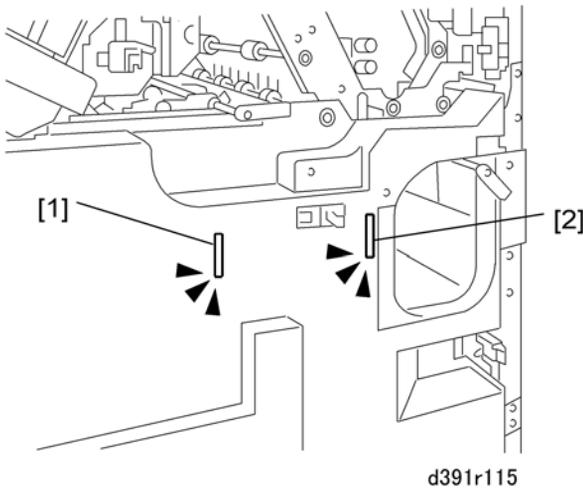
3. Insert piece of cardboard or folded piece of paper into the slots of the left [1] and right [2] door switches.
