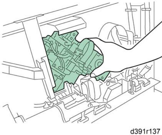
7. While holding the main gripper steady with one hand, remove the grip unit rotation motor.
