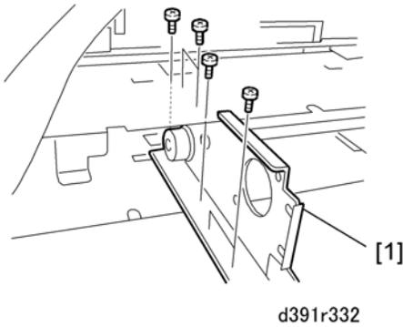
11. Remove the screws from the motor frame [1] (🔩 x6).
