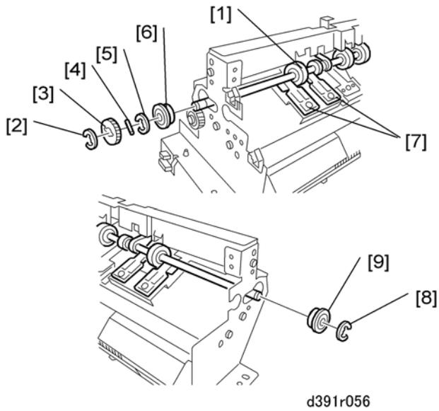
8. Remove the TE press roller unit [1].
