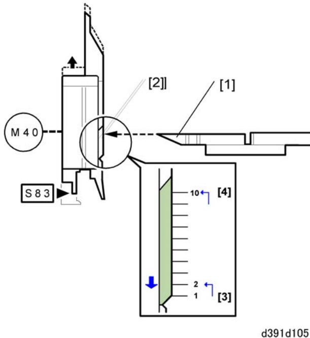
Cutting is performed by pushing the blade [1] against the blade cradle [2] with the edge of the book between the blade and cradle.
