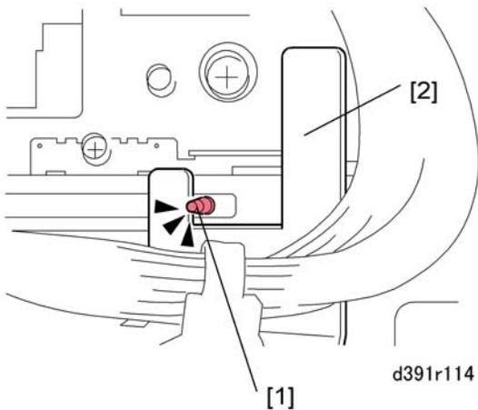
1. When reattaching the sensor plate confirm that the sensor pin [1] is positioned between the sides of the cutout [2] as shown above.
