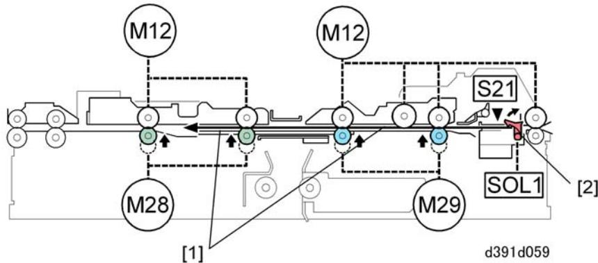
The spine fold motor: right (M29) on the right turns on, raises the two transport rollers on the right, and clamps the cover [1] in the roller nips.
