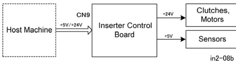
The bookbinder supplies power to the inserter (DC +5V, +24V). The DC +24V power is supplied to the clutches and motors. The DC +5V power goes to the sensors. Opening any cover of the inserter cuts the power supply, closing the cover restores the power supply.
