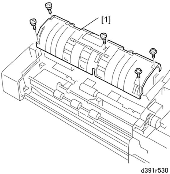
1. Remove the inserter rear cover. (☛ p.263)
