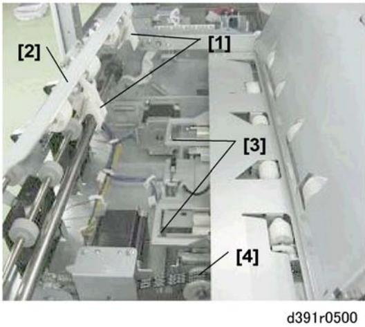
Make sure that the pressure arms [1] behind the exit unit [2] go through the holes of the left spine fold unit [3]. If this is difficult to do, turn the pulley [4] of the spine fold motor manually to move the left spine fold unit.
