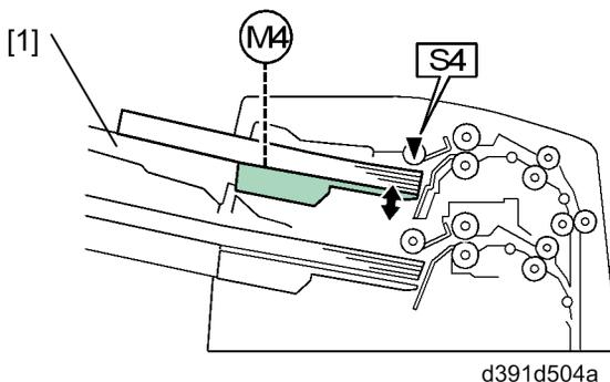
With paper loaded in the tray when the inserter receives a job start command from the bookbinder, the lift motor (M4 (INS)) for Tray A [1] turns on and raises the top tray until paper feed sensor (S4 (INS)) for Tray A detects the top of the paper stack and signals to stop the motor. Next, lift motor (M4 (INS)) reverses for a very brief time to lower the tray a short distance and then stops with the tray up and below the paper feed position.
