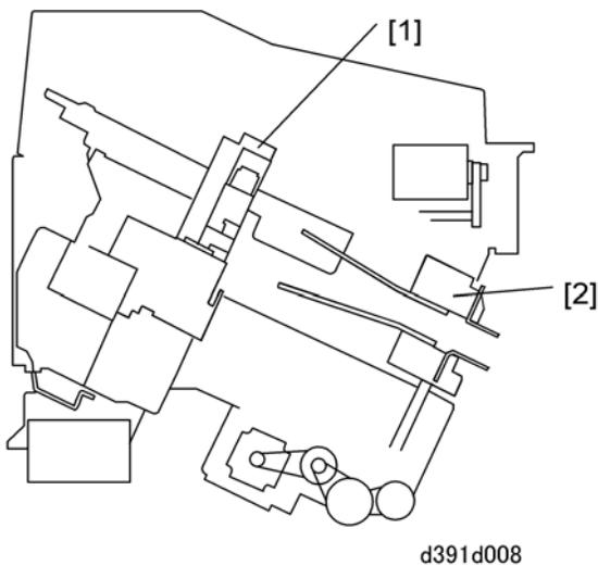
The sub grip unit [1] takes the aligned stack (signature) from the stacking tray unit and passes it to the main grip [2].
