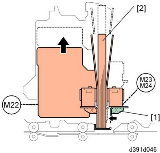
The gripper motor: front (M24) and gripper motor: rear (M23) switch on, close the main gripper [1], and clamp the signature [2]. The main grip lift motor (M22) turns on raises the grip unit and signature to the gluing position
