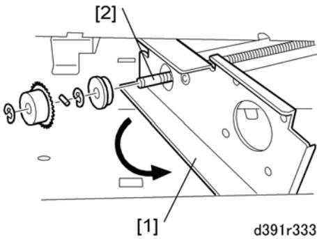
12. Move the motor frame [1] in the direction the arrow then remove the shaft [2] (🌀 x1, Sprocket x1, Lock pin x1, 🌀 x1, Bearing x1)
