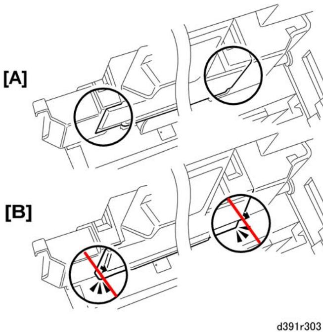
2. After the blade cradle has been reinstalled, at the front and rear confirm that blade cradle is aligned correctly [A] and not floating away [B] from or misaligned with the trimming unit.
