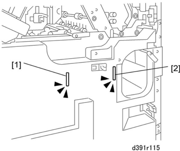
2. Insert piece of cardboard or folded piece of paper into the slot [1] of the left door switch and the slot [2] of the right door switch.
