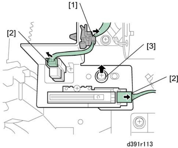
15. Remove the signature thickness sensor (S50)
