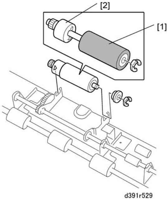
4. Remove the separation roller [1] (⌀ x1, Bushing x1)
