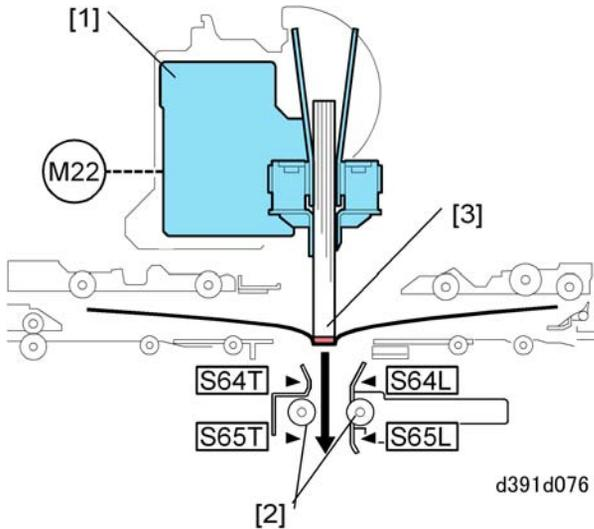
The main grip lift motor (M22) turns on and lowers the main grip unit [1] as far as the signature exit rollers [2]. Two sensor pairs in the signature transport path detect the presence of the joined cover and signature [3] as it is lowered:
