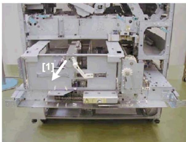
5. Pull out the trimming unit [1].
