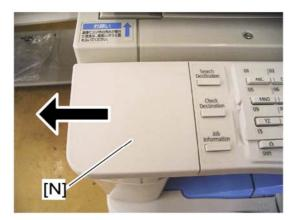
11. Remove the dummy cover [N] from the operation panel.
