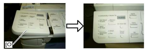
12. Install the fax operation panel [O] on the operation panel as shown.
