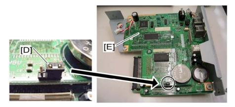
4. Switch the jumper switch [D] on the MBU [E] to "ON" position.
