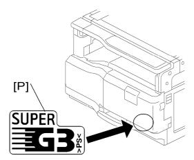
13. Attach the super G3 decal [P] to the front door as shown.
