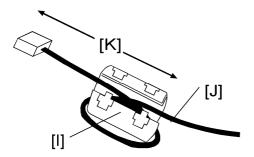
8. Attach the ferrite core [I] to the telephone cable [J]. The length [K] must be about 10 cm (4").
