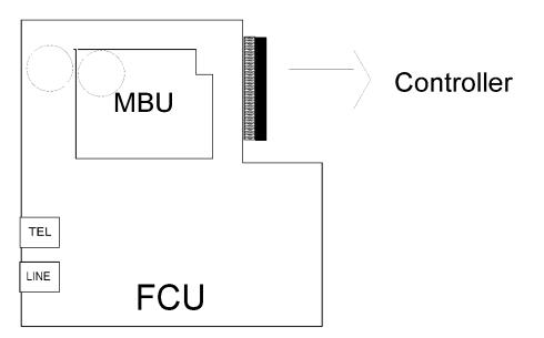
The basic fax unit consists of two PCBs: an FCU and an MBU.
