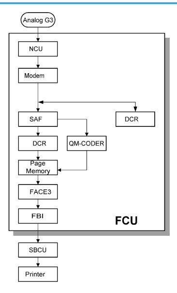
First, the FCU stores the incoming data from either an analog line to the SAF memory. (The data goes to the FACE3 at the same time, and is checked for error lines/frames.)
