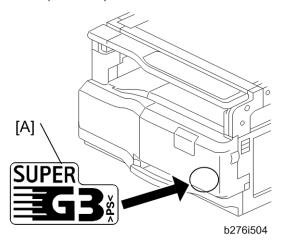
14. Attach the SG3 decal [A] to the front door as shown.
