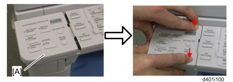
12. Install the fax operation panel [A] on the operation panel.
