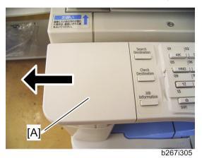
11. Remove the dummy cover [A] from the operation panel.
