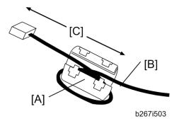
8. Attach the ferrite core [A] to the telephone cable [B]. The length [C] must be about 10 cm (4").
